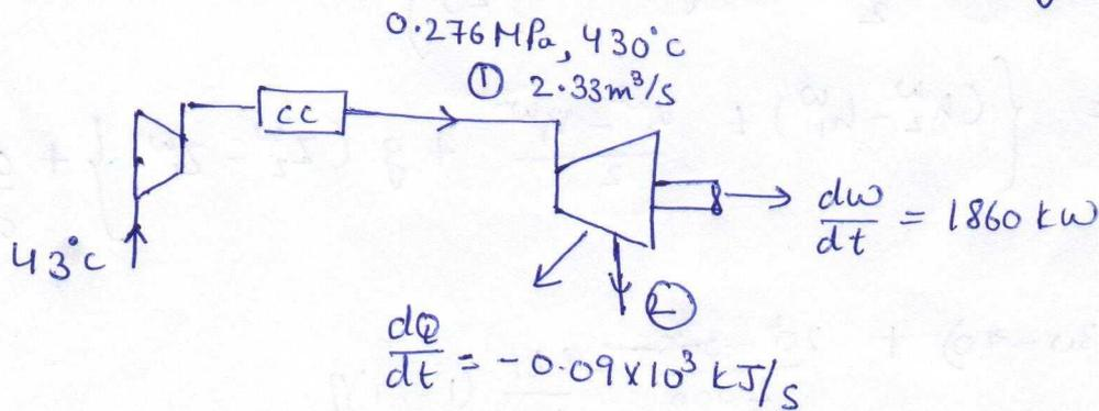
$$P_1 V_1 = m_1 R T_1 \Rightarrow \dot{m} = \frac{P_1 \dot{V}_1}{R T_1} = \frac{276 \times 2.33}{0.287 \times 316} = 7.091 \text{ kg/s}$$
