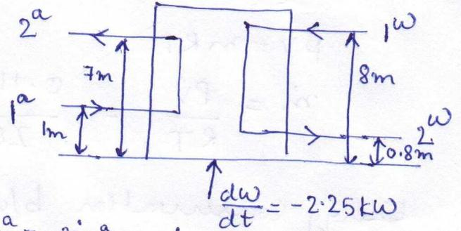
$$\dot{m}_1^a \left( h_1^a + \frac{V_1^{a2}}{2} + g z_1^a \right) + \dot{m}_1^w \left( h_1^w + \frac{V_1^{w2}}{2} + g z_1^w \right) + \frac{dQ}{dt}$$
